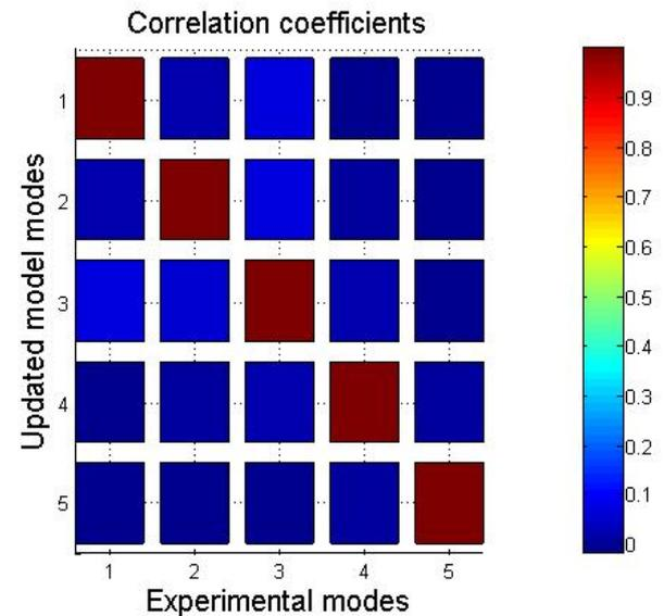
Fig. 6: Comparison of correlation matrix profile of experimental and model modes before and after updating
