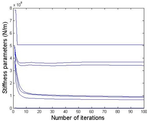
Fig. 5: Iteration histories of few representative stiffness parameters
