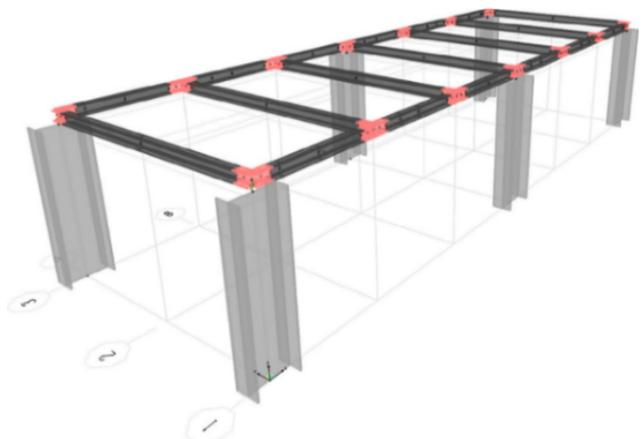
**Fig. 3: Finite Element model of the UCF benchmark structure in SAP2000**
