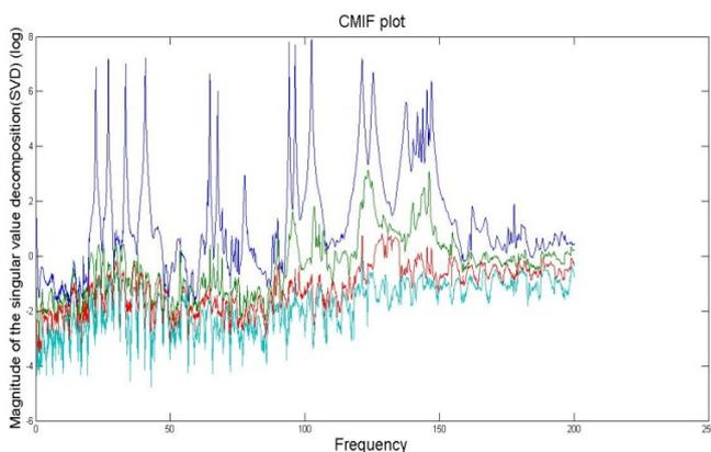
Fig. 4: Complex Mode Indicator Function (CMIF) plot
