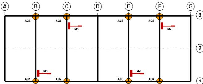
**Fig. 2: Accelerometer and impact locations for dynamic testing**
